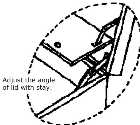
After painting, attach stay, lock, hinges, handle and so on. You can make a handle from a few of leather stuck together.
