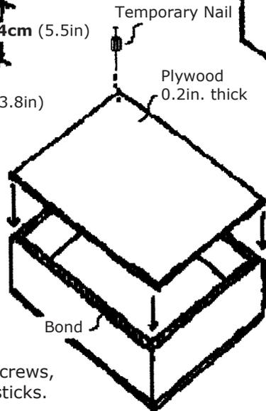
Attach plywood with bond on both side of a square frame. And temporarily nail it.
