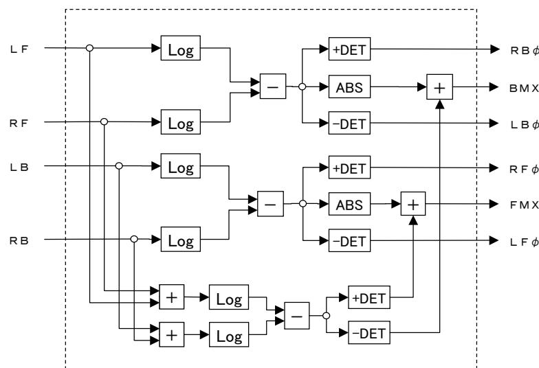
Direction detection Block Diagram
