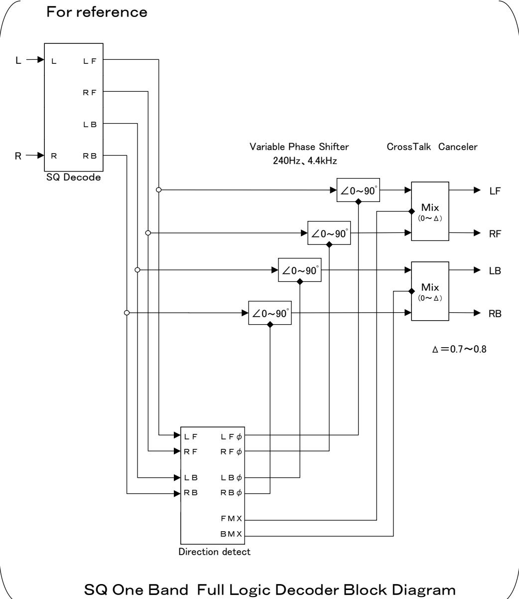
SQ One Band Full Logic Decoder Block Diagram
