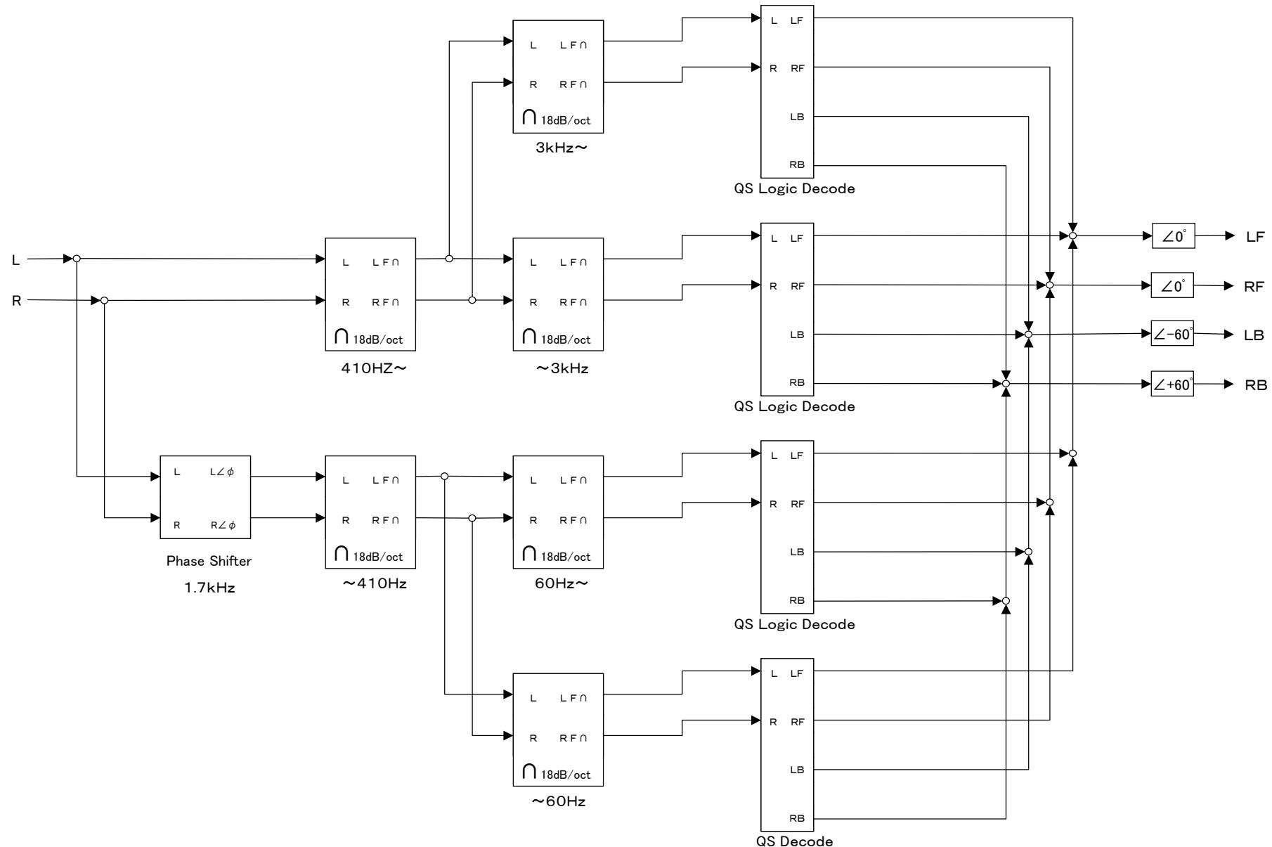
QS Three Band Full Logic Decoder Block Diagram
