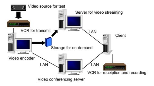
Figure A.1 – General configuration for measuement
